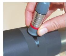
Do the second measurement by applying the probe on the anilox surface with the liquid.
