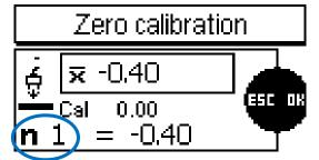
"n1" appears in the bottom left portion of the screen. It indicates that the first measurement is done.
