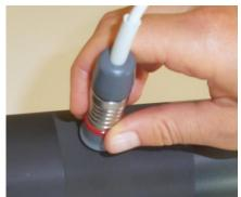
Do the *third* measurement by applying the probe on the anilox surface, without FerroFluid.
