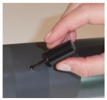
Apply the FerroFluid on the roll surface, in the form of a line about 1 cm long.
