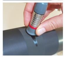
Do the third measurement by applying the probe on the anilox surface with the liquid.
