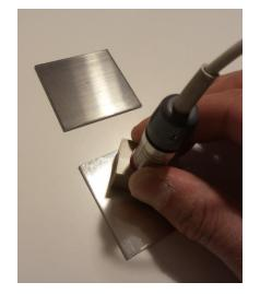
Apply the probe on the aluminum plate (light grey color).
