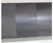
The measurement zone lies inside the circle. The probe has to be positioned in the circle.
