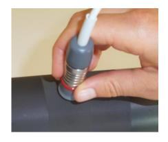
Do the *first* measurement by applying the probe on the anilox surface, without FerroFluid.
