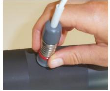
Do the second measurement by applying the probe on the anilox surface, without FerroFluid.
