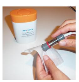
Clean the probe tip after the measurement, with the wipe provided in the kit.
