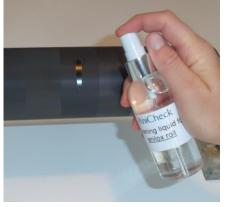
Clean the FerroFluid on the roll surface with the AniCheck cleaning fluid.
