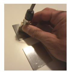
Apply the probe on the steel plate (dark grey color).
