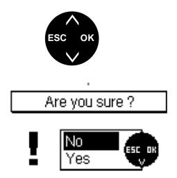
A measurement can be interrupted at any time by pressing ESC.
