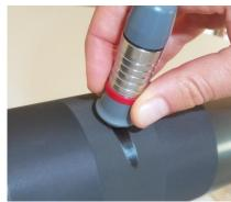
Do the first measurement by applying the probe on the anilox surface with the liquid.
